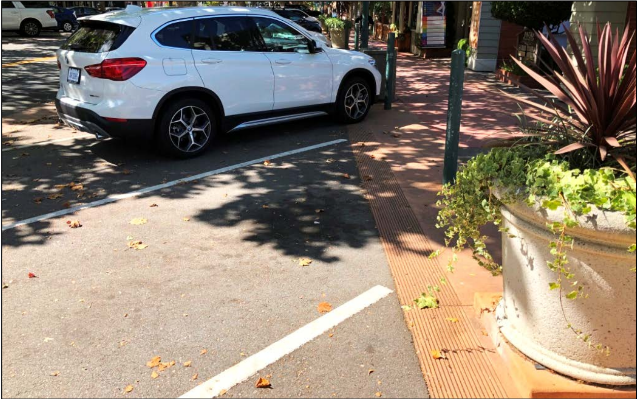
Photo 8 – City of Novato’s revitalized “Old Town” district: structural bollards, lamp poles, and planters prevent vehicular encroachment into the accessible public sidewalks.
