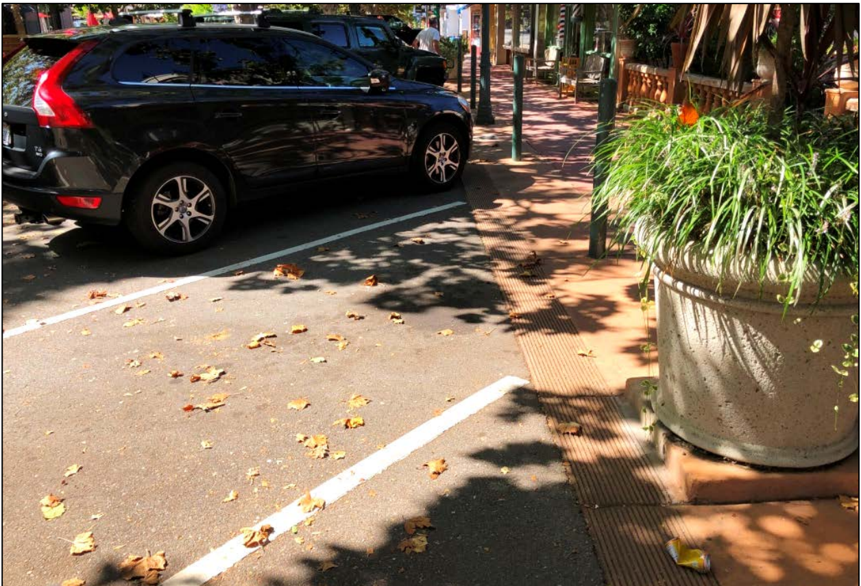
Photo 9 – City of Novato’s revitalized “Old Town” district: structural bollards, lamp poles, and planters prevent vehicular encroachment into the accessible public sidewalks.
