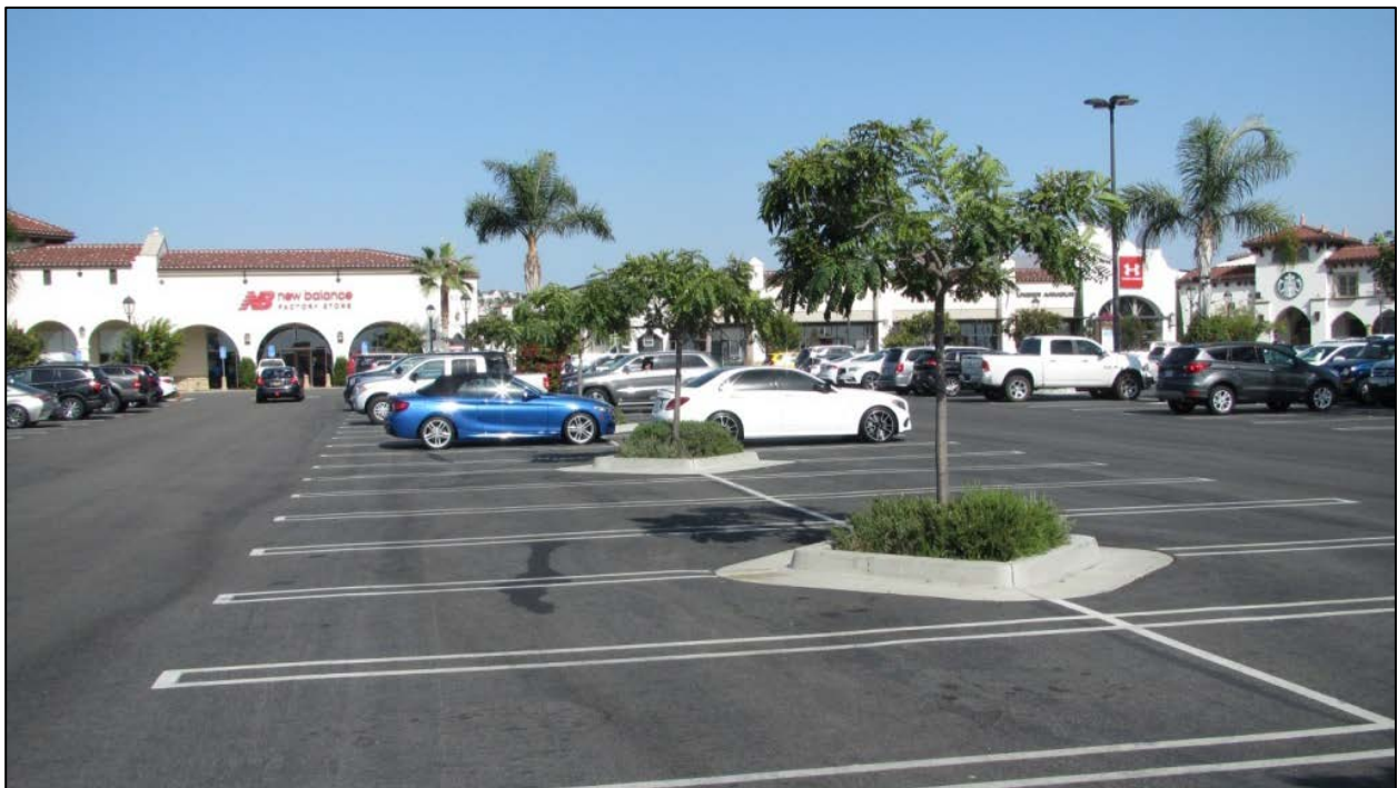
Photo 6 – The large parking lot in Southern California was designed and constructed without wheel stops, which are potential tripping hazards (and which are not required by state or federal laws, codes, or regulations).
